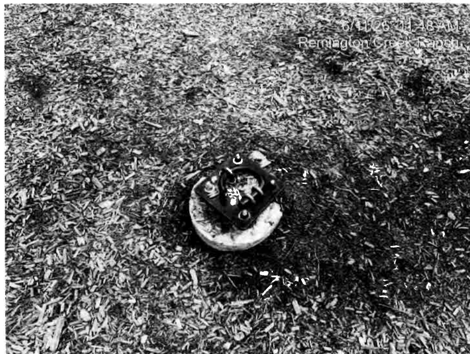
Remington Creek Ranch Playground – broken spring toy
